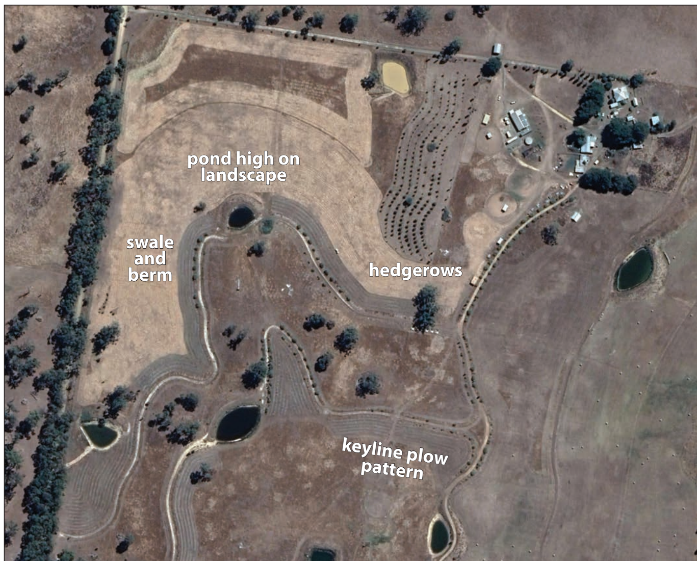
Figure 1.4. The photograph shows an aerial view of Taranaki Farms showing examples of Keyline Design as labeled.
